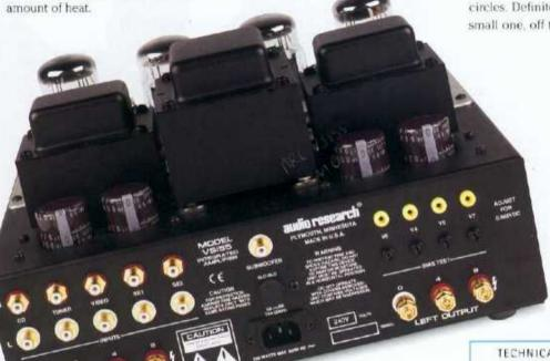
Obviously, the valves get fairly warm, but less predictably so too does the mains transformer and (to a much lesser degree) the two output transformers. With the latter, the rise in temperature is almost certainly down to heat conduction from the four output tubes and mains transformer. Certainly, after the amp's been on a couple of hours or more, the whole case warms up.
